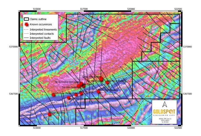
Figure 1 - Interpreted lineaments, contacts and faults in Wilding and East-Alder properties, over reduced to pole magnetics.
