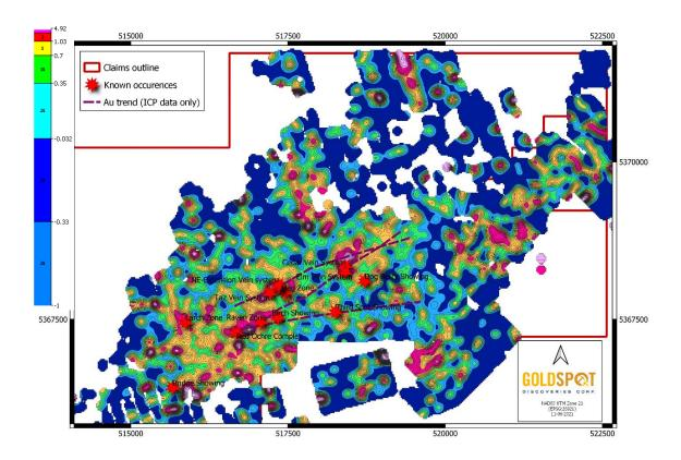
Figure 2 – Levelled gold in soils grid using IDW interpolation method. Levelling geochemical data creates a unitless ratio, so values on the legend <u>do not</u> represent ppm, ppb, etc.
