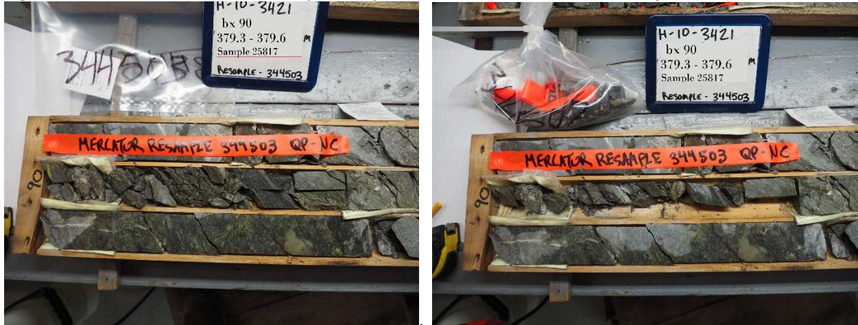
Figure 12-9: Quarter-core check sample completed for drill holes H-10-3421 (April, 2021)
